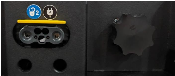
Figure 33 Pendant and manual charge port bay lock-out/tag-out
