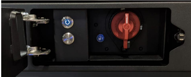
Figure 32 Lock-out/tag-out bay lock-out OFF position
