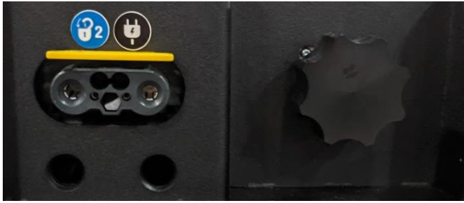
Figure 26 Pendant and manual charge port bay lock-out/tag-out
